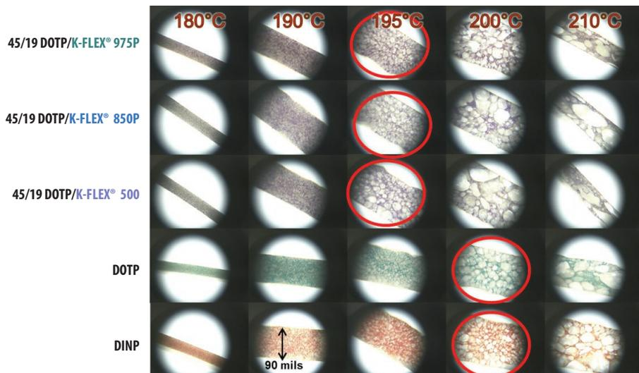
**Figure 2. Blow oven temperature can be reduced by a minimum of 2.5% while improving foam quality when expanding back foams formulated with blends of K-FLEX® and DOTP.**
