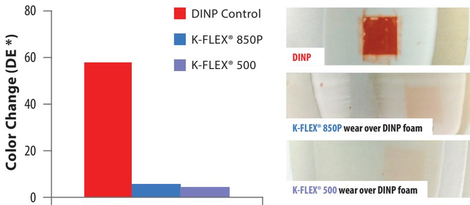
**Figure 1. Wear/clear layer stain resistance to oil brown traffic stainant.** The wear layers were applied over 100% DINP foam layers and demonstrate excellent stain resistance and protection of the construct.
