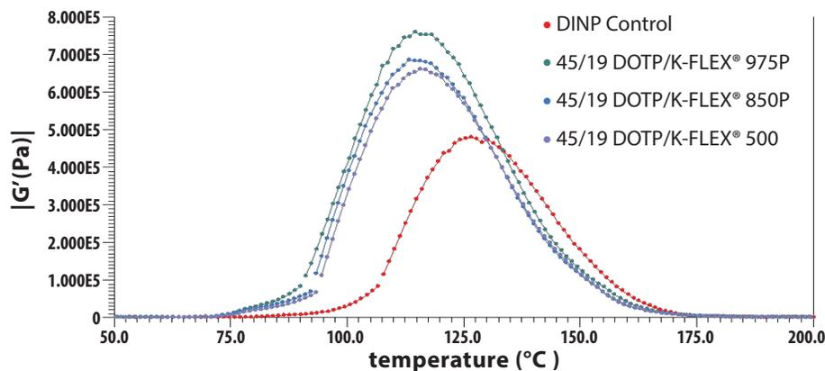
**Figure 4. Gelation onset temperature occurs at 10-20 °C lower temperature than GP plasticizers when using blends of K-FLEX® with DOTP in this back foam formulation.**
