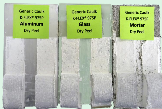
K-FLEX® 975P tested in an ASTM C920 latex caulk over aluminum, glass, and mortar substrate.
